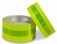
Reflexite® FTP2000 is a thin and flexible monolayered fluorescent lime retroreflective fire tape designed to meet or exceed the requirements of EN 469:2005 Protective Clothing for Fire-Fighters offering superior reflectivity and durability under today's most demanding fire-fighting conditions.
